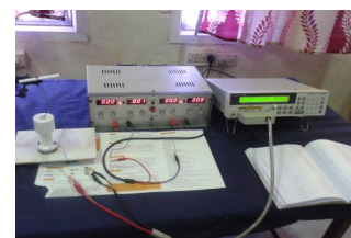
LCR Meter (Agilent 4263B)
