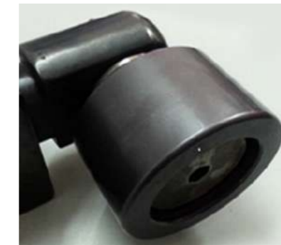
WC ROLLER BEFORE COATING
