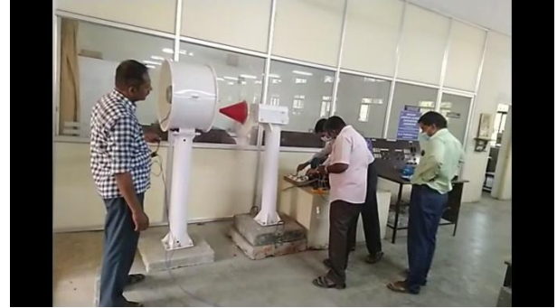
500W Wind turbine Emulated PMSG power generator
