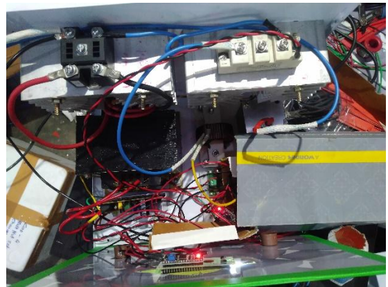
Hardware Fabrication of 500W PV Emulator
