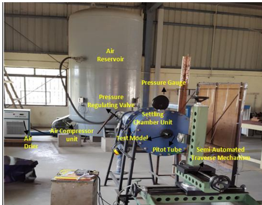
High-speed free jet facility at the Department of Aeronautical Engineering, Rajalakshmi Engineering College
